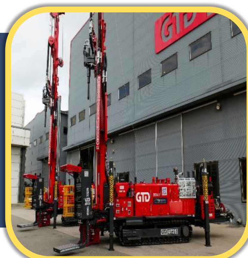
TRACK MOUNTED RIG
